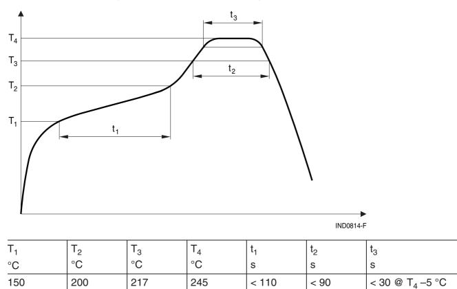
Time from 25 °C to  $T_4$ : max 300 s Maximal numbers of reflow cycles: 3
