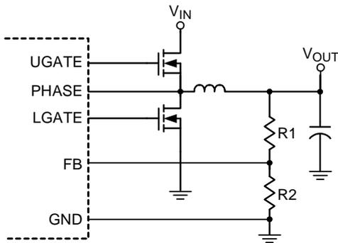
Figure 4. Setting VOUT with a Resistor Divider
