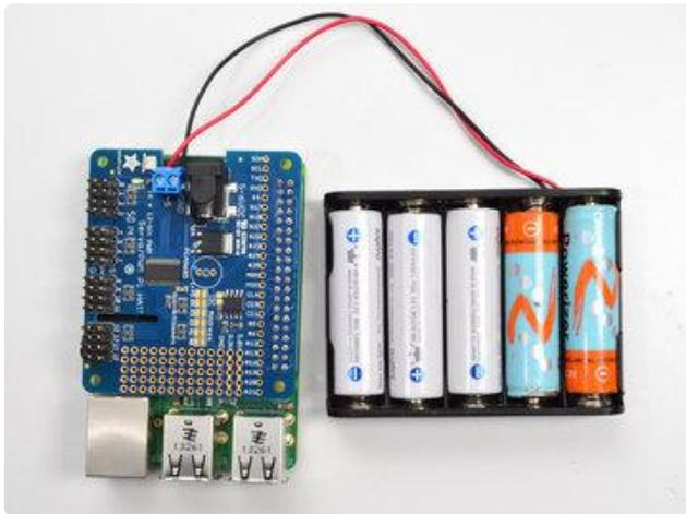
Or, for portable use, a 4 or 5 x AA battery pack can be connected to the terminal block.
