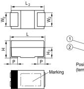
Positive pole marking (terminal slot optional)
