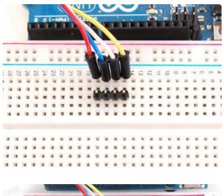
Now you're ready to wire it up to a microcontroller. We'll assume you want to use a 4pin header. You can also of course solder wires directly. Place a 4-pin piece of header with the LONG pins down into the breadboard.
