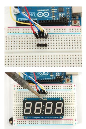
Now you're ready to wire it up to a microcontroller. We'll assume you want to use a 4pin header. You can also of course solder wires directly. Place a 4-pin piece of header with the LONG pins down into the breadboard.
