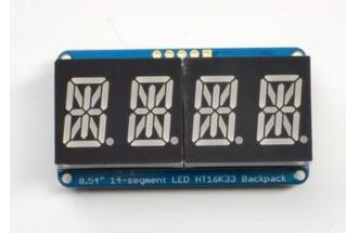
Remove the parts from packaging and place the LED matrices OVER the silkscreen side. DO NOT PUT THE DISPLAY ON UPSIDE DOWN OR IT WONT WORK!! Check the image below to make sure the 'decimal point' dots are on the bottom, matching the silkscreen.
