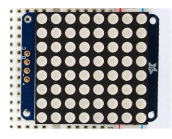
The default orientation for graphics commands on this display places pixel (0,0) at the top-left when the header is at the left and Adafruit logo at the right. To use the matrix as shown above (header at top, logo at bottom), call matrix.setRotation(3) before issuing graphics commands.
