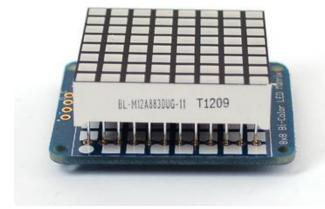
Remove the parts from packaging and place the LED matrix OVER the silkscreen side.
