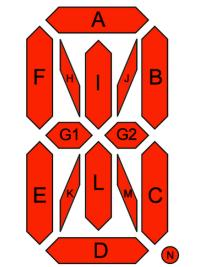
The bitmask is a 16-bit number that can be passed in as a single Hexidecimal, Decimal, or binary number. It can also be passed in as a list or tuple containing 2 separate 8-bit numbers. Here are some of the ways to set the digits. All of these different methods create a box with an X in the center:
