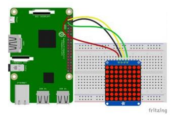
Raspberry Pi 3.3V to LED Matrix VIN Raspberry Pi GND to LED Matrix GND Raspberry Pi SCL to LED Matrix SCL Raspberry Pi SDA to LED Matrix SDA
