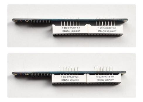
To keep the two bargraphs lined up nicely, you can use a little masking or scotch tape on the bargraph modules, tape them so they are in a straight line. There is a little play during soldering so if you don't do this the two modules may not be in a perfect line.
