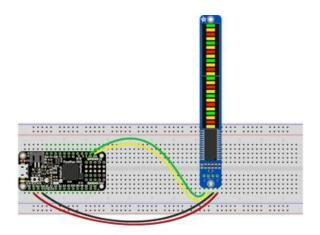
Microcontroller 3V to Bargraph VIN Microcontroller GND to Bargraph GND Microcontroller SCL to Bargraph SCL Microcontroller SDA to Bargraph SDA
