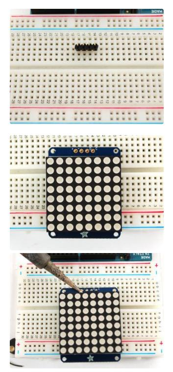
Now you're ready to wire it up to a microcontroller. We'll assume you want to use a 4pin header. You can also of course solder wires directly. Place a 4-pin piece of header with the LONG pins down into the breadboard.
