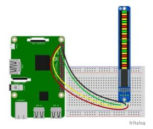
Raspberry Pi 3.3V to Bargraph VIN Raspberry Pi GND to Bargraph GND Raspberry Pi SCL to Bargraph SCL Raspberry Pi SDA to Bargraph SDA
