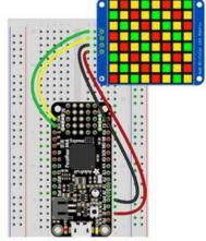
Microcontroller 3V to LED Matrix VIN Microcontroller GND to LED Matrix GND Microcontroller SCL to LED Matrix SCL Microcontroller SDA to LED Matrix SDA
