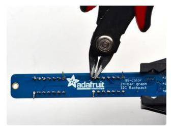
Once soldered, clip each pin. They're quite short and the pins are thicker than usual, so do this over/inside a trash bin so that the pins don't fly off and it you or your pets.
