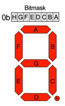
The bitmask is a single 8-bit number that can be passed in as a single Hexidecimal, Decimal, or binary number. This will use a couple different methods to display **8.8.EE**:
