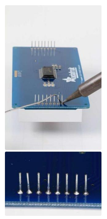
Then solder each pin. There are 8 on each end for a total of 16.
