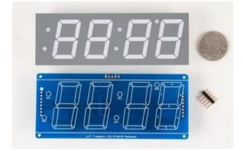
When you buy a pack from Adafruit, it comes with the fully tested and assembled backpack as well as a 7-segment display in one of the colors we provide (say, red, yellow, blue or green). You'll need to solder the matrix onto the backpack but its an easy task.
