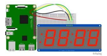
Raspberry Pi 3.3V to 7-Segment Display IO Raspberry Pi 5V to 7-Segment Display VIN Raspberry Pi GND to 7-Segment Display GND Raspberry Pi SCL to 7-Segment Display SCL Raspberry Pi SDA to 7-Segment Display SDA
