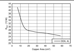
Figure 9-3. Typical  $R_{\theta JA}$  versus Copper Area for a Four-Layer Board
