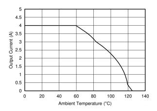
Figure 9-4. Maximum Output Current versus Ambient Temperature V<sub>IN</sub> = 12 V, V<sub>OUT</sub> = 5 V, R<sub> $\theta$ JA</sub> = 30°C/W,  $f_{SW}$  = 400 kHz
