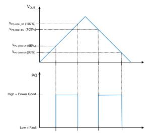
Figure 8-1. Static Power-Good Operation
