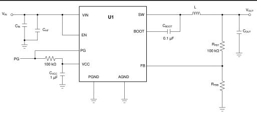
Figure 9-21. Circuit for Application Curves
