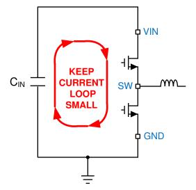
Figure 11-1. Current Loops with Fast Edges
