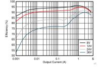
Efficiency versus Output Current  $V_{OUT}$  = 5 V, 400 kHz, HSOIC
