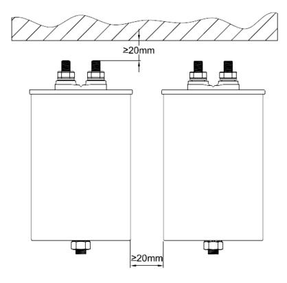
Figure 5: Installation space requirements
