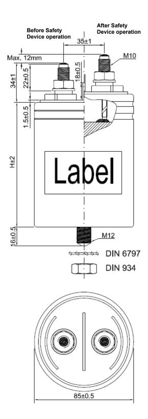
**Figure 4:** Series B32362 (D = 85 mm)
