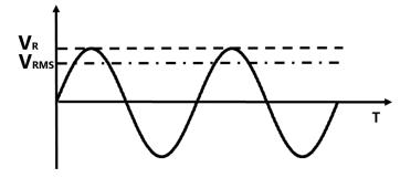
Figure 9: Voltage V<sub>RMS</sub>
