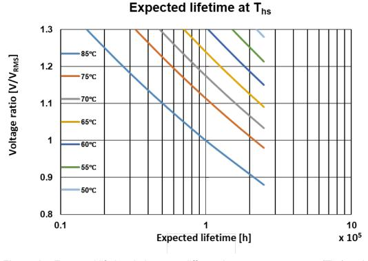
Figure 15: Expected lifetime in hours at different hotspot temperatures (Ths) and voltages V<sub>RMS</sub>.
