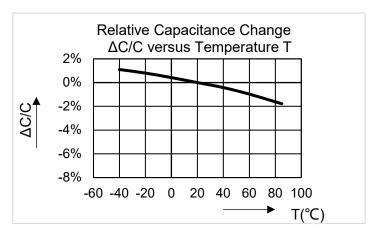
Figure 8: Temperature dependence of capacitance
