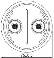
**Figure 3:** Series B32362 (D = 75 mm)
