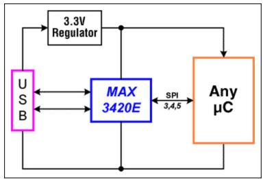
Figure 1. A USB bus-powered widget.
