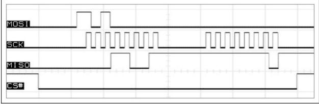
Figure 4. SPI interface operating in mode (0,0).
