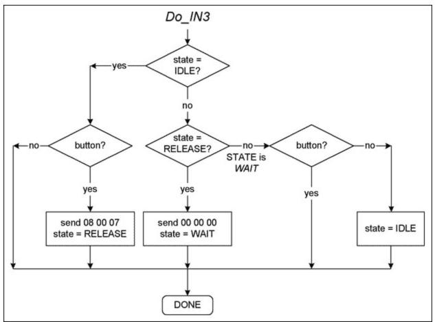
Figure 7. Flow diagram of the panic button.
