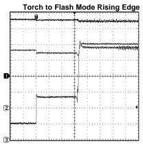
$V_{\text{IN}}$  = 3.6V, Load = 200mA/800mA (Torch/Flash), LED = PWF1 CH1 (TOP):  $V_{\text{IN}}$ ; Scale: 1V/Div, DC Coupled CH2 (MIDDLE):  $V_{\text{OUT}}$ ; Scale: 1V/Div, DC Coupled
