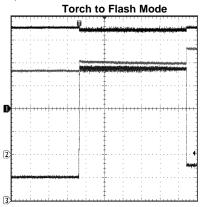
$\label{eq:VIN} $V_{IN}=3.6$V, Load = 200mA/800mA (Torch/Flash), LED = PWF1; CH1 (TOP): $V_{IN}$; Scale: 1V/Div, DC Coupled CH2 (MIDDLE): $V_{OUT}$; Scale: 1V/Div, DC Coupled CH3 (BOTTOM): $I_{IN}$; Scale: 200mA/Div Time scale: 100ms/Div$
