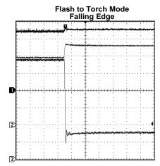
V<sub>IN</sub> = 3.6V, Load = 800mA/200mA (Flash/Torch), LED = PWF1
