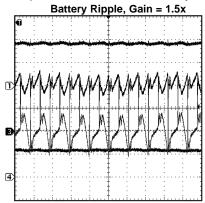
$$\begin{split} &V_{\text{IN}} = \text{Li-Ion Battery at 3.7V, Load} = 400\text{mA, LED} = \text{PWF1;} \\ &\text{CH1 (MID-TOP): } &V_{\text{OUT}}; \text{ Scale: } 20\text{mV/Div, AC Coupled;} \\ &\text{CH2 (MID-BOTTOM): } &V_{\text{IN}}; \text{ Scale: } 50\text{mV/Div, AC Coupled;} \end{split}$$
