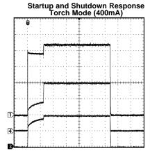
V<sub>IN</sub> = 3.6V, Load = 400mA, LED = PWF1; CH1 (TOP): V<sub>OUT</sub>; Scale: 1V/Div, DC Coupled;
