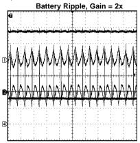
$V_{IN}$  = Li-Ion Battery at 3.7V, Load = 400mA; LED = PWF1; CH1 (MID-TOP):  $V_{OUT}$ ; Scale: 20mV/Div, AC Coupled; CH2 (MID-BOTTOM):  $V_{IN}$ ; Scale: 50mV/Div, AC Coupled; CH3 (TOP):  $V_{IN}$ ; Scale: 1V/Div, DC Coupled; CH4 (BOTTOM):  $I_{IN}$ ; Scale: 500mA/Div; Time scale: 1 $\mu$ s/Div
