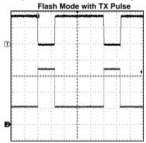
$V_{\text{IN}} = 3.6\text{V}$ , Load = 700mA (Flash), LED = PWF1 CH1 (TOP):  $V_{\text{TX}}$ ; Scale: 1V/Div, DC Coupled CH2 (BOTTOM):  $I_{\text{LED}}$ ; Scale: 200mA/Div
