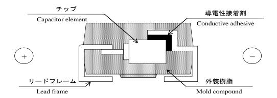
Lead frame base : Iron-Nickel alloy/Copper plating
