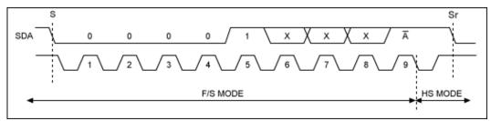
Figure 1. These waveforms represent a transfer from Standard- or Fast-mode I<sup>2</sup>C to Hs mode.
