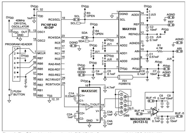
Figure 2. The I<sup>2</sup>C peripheral internal to this PIC18F442 μC connects to a 16-bit ADC (MAX1169).
