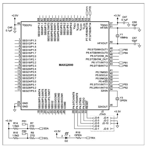
Figure 3. This schematic (based on the MAXQ2000 low-power LCD  $\mu$ C) depicts an  $l^2$ C master capable of operating in Standard, Fast, or Hs mode.
