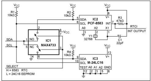
Figure 1. A dual analog switch (IC1, the MAX4733) and a single controller line (SELECT) enable this I<sup>2</sup>C bus to select between two peripherals with identical addresses.
