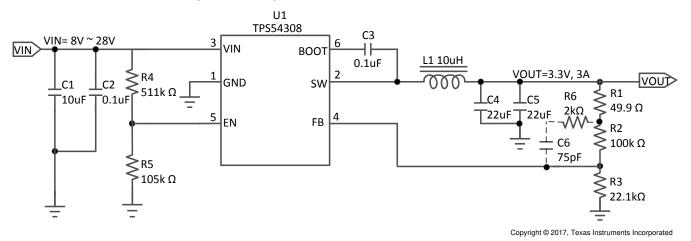
Figure 8-1. 5-V, 3-A Reference Design
