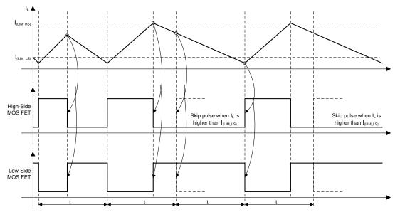
Figure 7-2. Overcurrent Protection for Both MOSFETs
