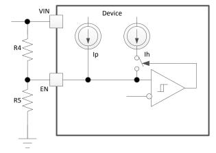
Figure 7-1. Adjustable VIN Undervoltage Lockout
