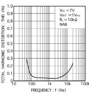
Fig.5 Total harmonic distortion vs. frequency
