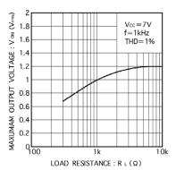
Fig.13 Maximum output voltage vs. load resistance
