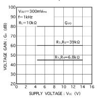
Fig.6 Voltage gain vs. supply voltage
