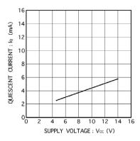
Fig.2 Quiescent current vs. power supply voltage
