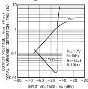
Fig.11 Input/output characteristics
