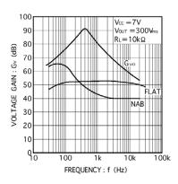
Fig.4 Voltage gain vs. frequency
