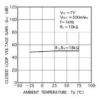
Fig.7 Closed loop voltage gain vs. ambient temperature
