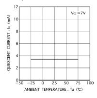
Fig.3 Quiescent current vs. ambient temperature
