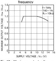
Fig.12 Maximum output voltage vs. power supply voltage
