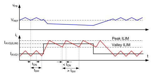
Figure 11. Current Limit Timing Diagram
