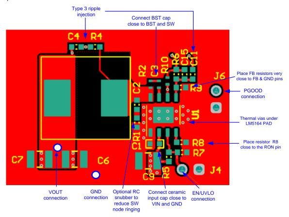
Figure 28. LM5164 Single-Sided PCB Layout Example
