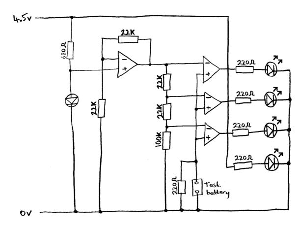
Comparators are used to compare one signal to another. They have two inputs: one labelled with a '-' and the other with a '+'. If the voltage on the '+' input is greater than that on the '-', then the output (the point of the triangle) will be 4.5V. If the signal on the '-' input is larger than the '+' input, then the output becomes zero.
