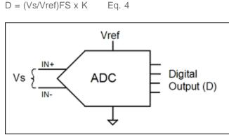
Figure 2. Generic analog-to-digital converter.
