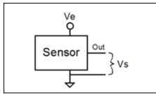
Figure 1. Generic ratiometric sensor.
