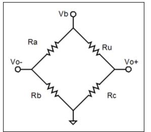
Figure 9. Illustration of a Wheatstone bridge which is comprised of two voltage-dividers powered from the same voltage source.
