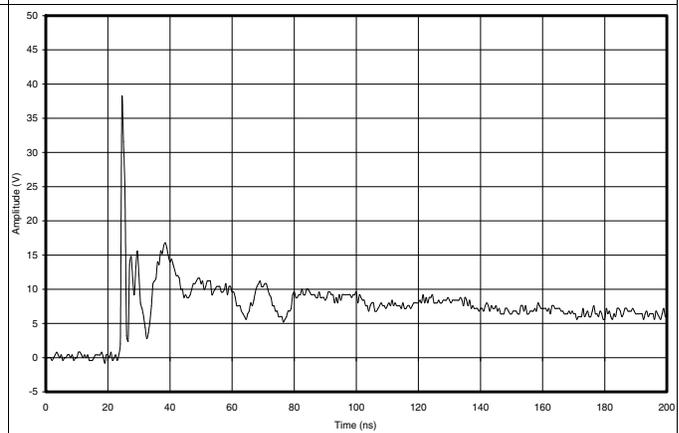
Figure 4. IEC Clamping Waveforms 8-kV Contact, 1-GHz Bandwidth
