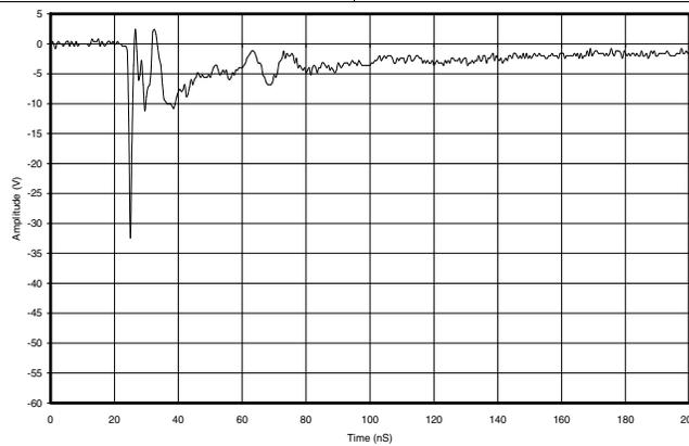
Figure 5. IEC Clamping Waveforms -8-kV Contact, 1-GHz Bandwidth
