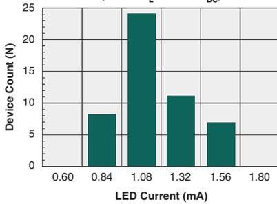
Typical I<sub>F</sub> for Switch Dropout
