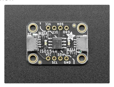
Sometimes you'll find yourself with an I2C bus controller on one side, and an I2C bus device on the other and you gotta keep em (electrically) separated (). Maybe because one is Earth-grounded, maybe because you've got some funky power monitoring setup, maybe you want to reduce noise.
