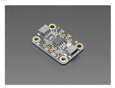
Usage is easy - you get power/ground/clock/data breakout pads for each side as well as a matching STEMMA QT connector. Unlike our other QT boards, the two sides are obviously electrically isolated, which means each half must be powered! Check that the green LED is lit on both sides. Now send data over I2C and you're good to go. We have 10K pullups on each side, from the I2C pins to the matching VCC for that side.
