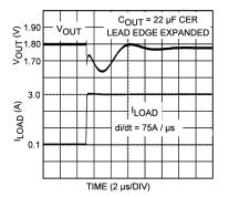
Figure 18. 22-µF Ceramic Output Capacitor
