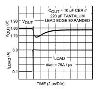
Figure 21. 10-µF Ceramic Paralleled by 220-µF Tantalum
