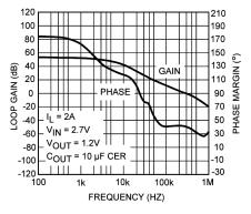
Figure 13. Gain-Bandwidth Plot for 2-A Load
