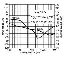
Figure 14. Gain-Bandwidth Plot for No Load
