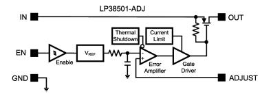
Figure 11. LP38501-ADJ Block Diagram
