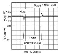
Figure 15. Load Transient Response: 10-µF Ceramic, 0.5-A/µs Di/Dt
