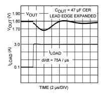
Figure 19. 47-µF Ceramic Output Capacitor
