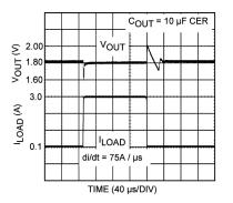
Figure 16. Load Transient Response: 10-µF Ceramic, 75 A/µs di/dt
