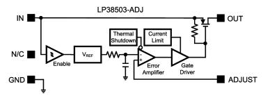
Figure 12. LP38503-ADJ Block Diagram
