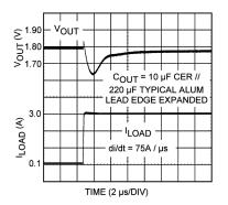
Figure 20. 10-µF Ceramic Paralleled by 220-µF Generic Aluminum Electrolytic
