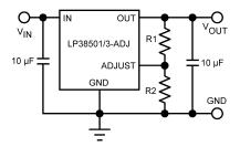
Figure 25. Setting Output Voltage
