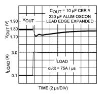
Figure 22. 10-µF Ceramic Paralleled by 220-µF OSCON
