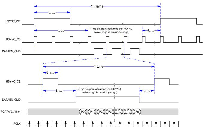
Figure 5. Parallel Interface Frame Timing
