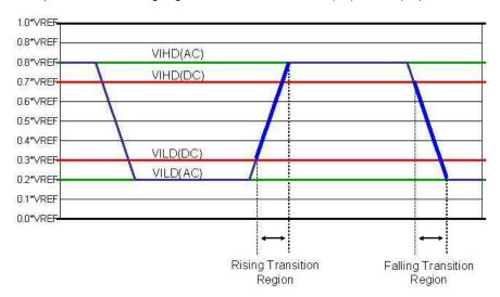
Figure 2. Low Speed (Ls) I/O Input Thresholds
