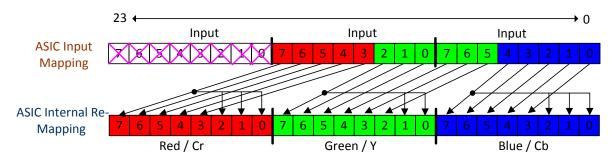
Figure 10. 16-Bit Rgb-565 I/O Mapping
