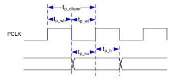
Figure 6. Parallel Interface General Timing
