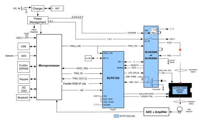
Figure 13. Typical Application Diagram
