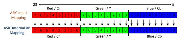
Figure 9. 24-Bit Rgb-888 I/O Mapping
