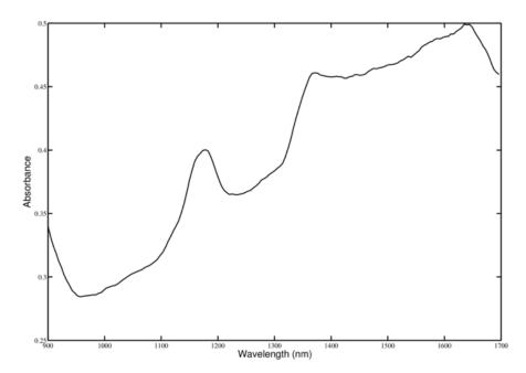
Figure 14. Sample DLPC150-Based Spectrometer Output
