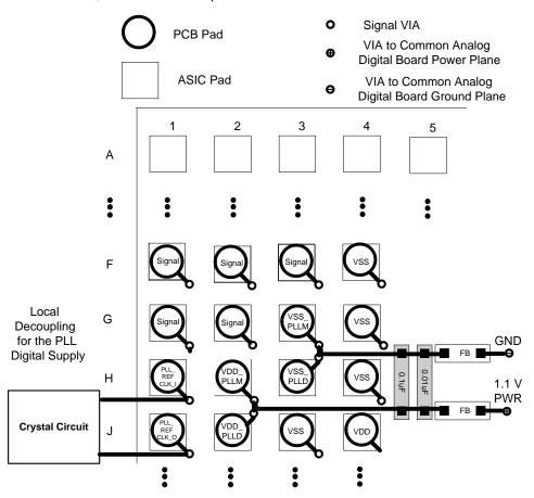
Figure 17. PLL Filter Layout
