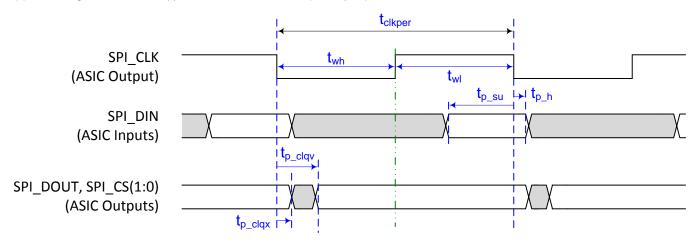
Figure 7. Flash Interface Timing
