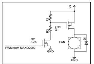
Figure 2. A possible hardware setup for connecting the PWM output to the fan.
