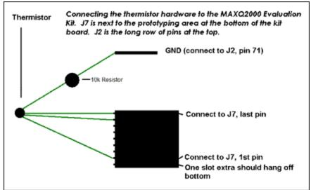
Figure 1. Connection of the thermistor hardware to the MAXQ2000 evaluation kit.
