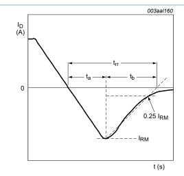
Fig. 16. Reverse recovery timing definition
