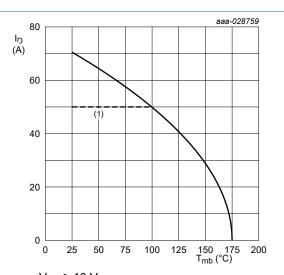
$V_{GS} \ge 10 \text{ V}$  (1) 50A continuous current has been successfully demonstrated during application tests. Practically the current will be limited by PCB, thermal design and operating temperature.
