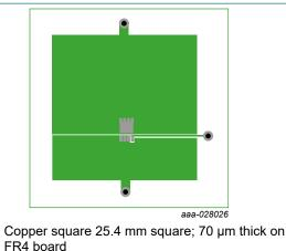
Fig. 5. PCB layout for resistance from junction to ambient
