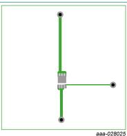
70 µm thick copper on FR4 board
