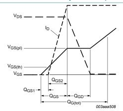
Fig. 13. Gate charge waveform definitions
