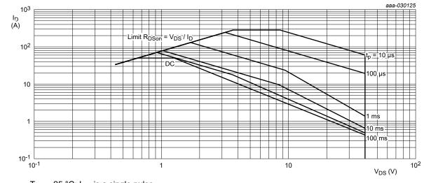
$T_{mb}$  = 25 °C;  $I_{DM}$  is a single pulse
